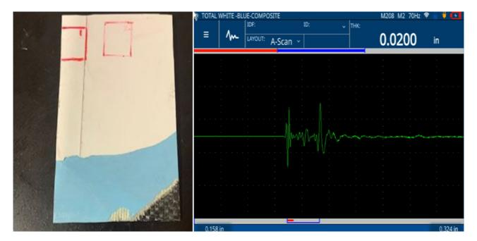
**Individual layer thickness**: In this measurement, the 20 MHz transducer and ultrasonic setup are optimized to amplify the echoes for each of the three layers of the coating on the composite. The coating includes a surfacer layer and two topcoat layers.
